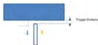
Picture : Proximity sensor triggering distances assessment(Bottom edge)
