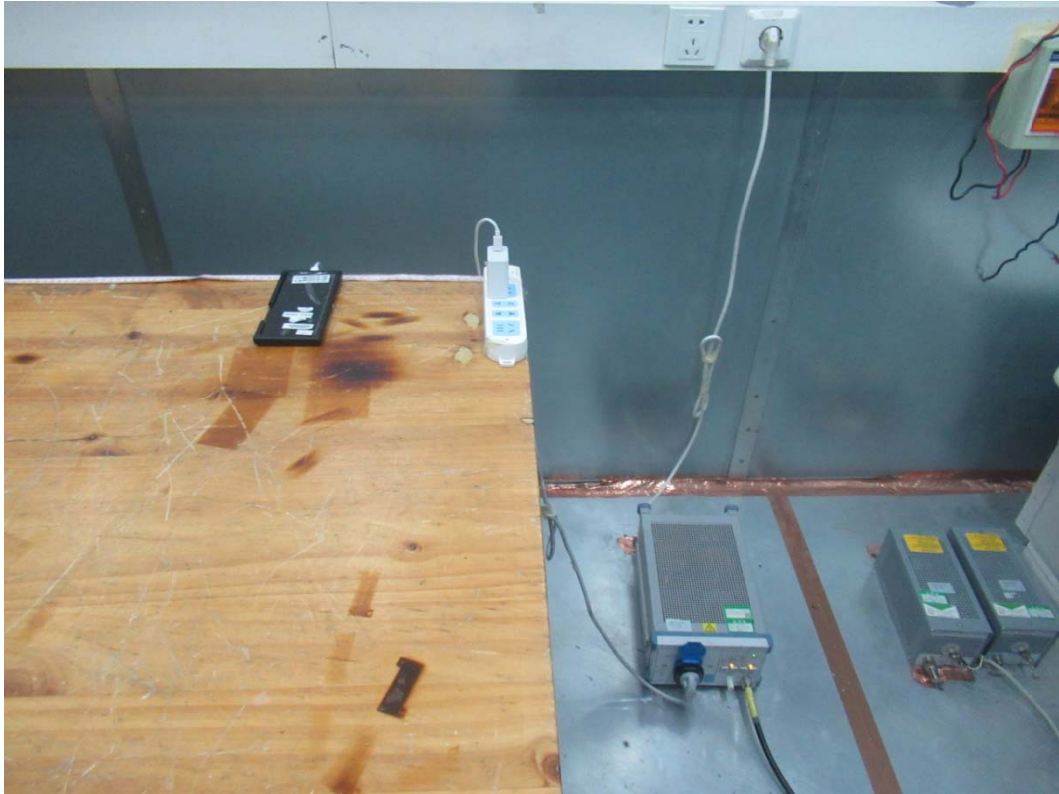
Picture 2 Conducted Emission Test Setup
