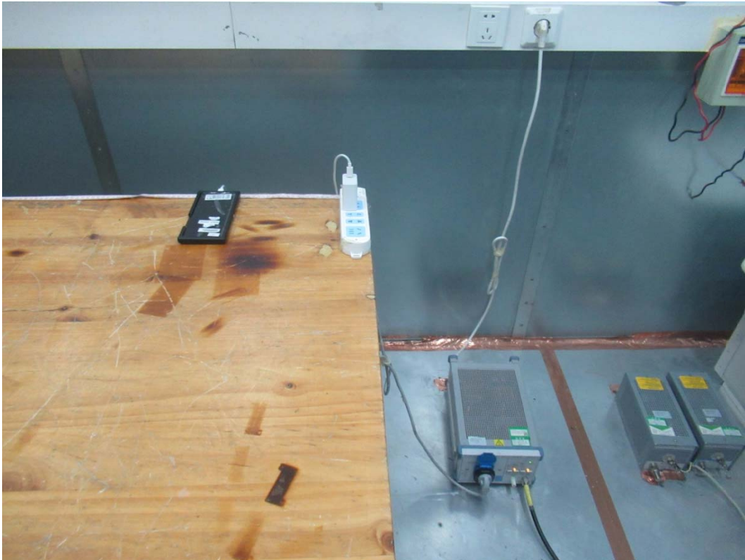
Picture 2: Conducted Emissions Test Setup
