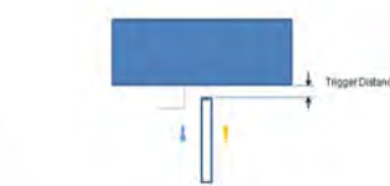
Picture: Proximity sensor triggering distances assessment (Bottom edge)
