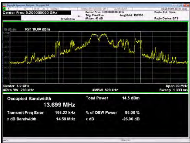
U-NII-1, 802.11ax HE20 MU Mode 26-Tones, Carrier frequency (MHz): 5200
