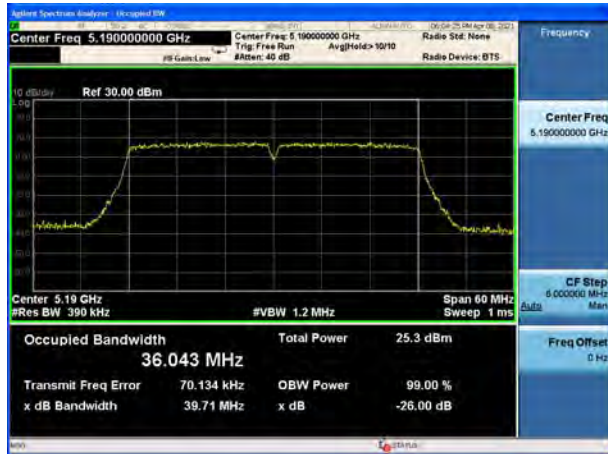
U-NII-1, 802.11n HT40 Carrier frequency (MHz): 5230
