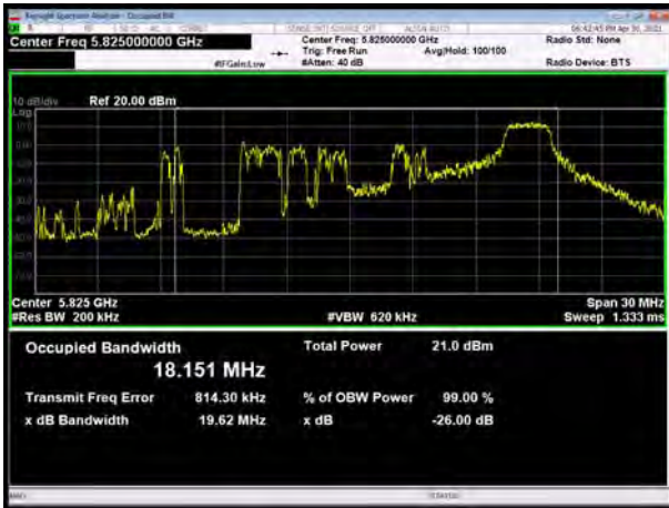
U-NII-3, 802.11ax HE20 MU Mode 26-Tones, Carrier frequency (MHz): 5825
