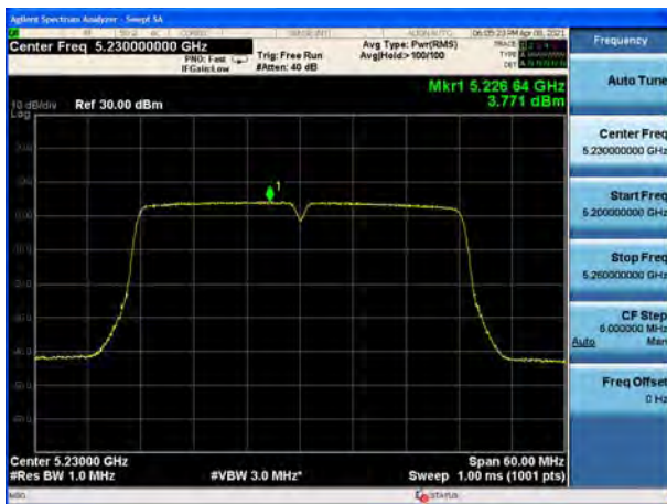
U-NII-1, 802.11ac VHT40, Channel No.: 38
