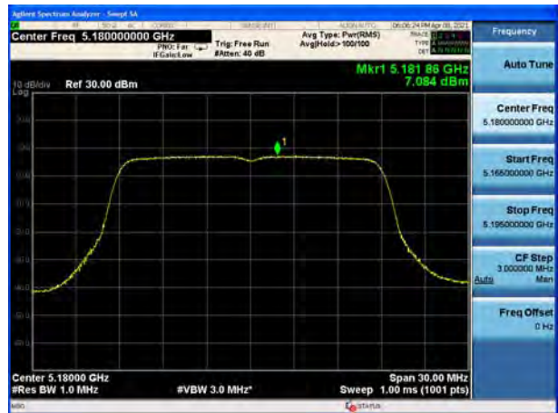
U-NII-1, 802.11ac VHT20, Channel No.: 40
