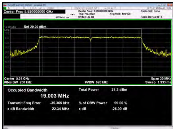
U-NII-2C, 802.11ax HE20 SU Mode 242-Tones, Carrier frequency (MHz): 5700
