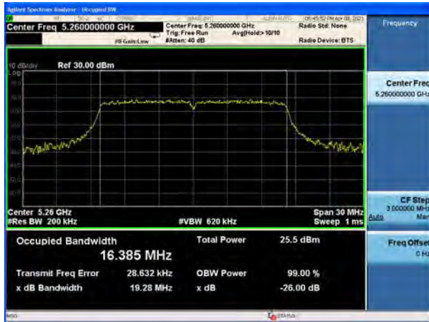
U-NII-2A, 802.11a Carrier frequency (MHz): 5300
