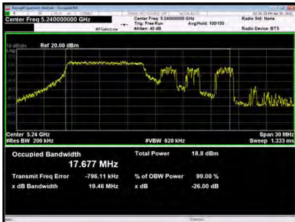
U-NII-1, 802.11ax HE40 SU Mode 484-Tones, Carrier frequency (MHz): 5190
