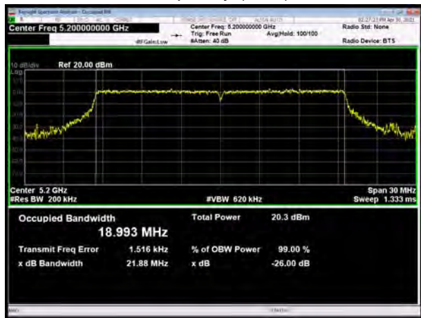
U-NII-1, 802.11ax HE20 SU Mode 242-Tones, Carrier frequency (MHz): 5200
