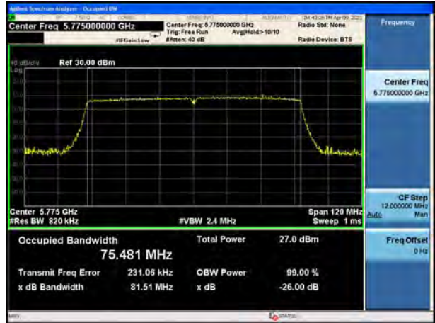
U-NII-3, 802.11ax HE40 Carrier frequency (MHz): 5755
