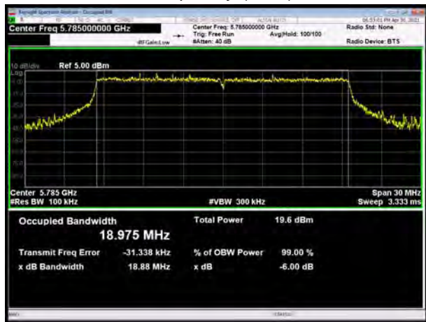
U-NII-3, 802.11ax HE20 SU Mode 242-Tones, Carrier frequency (MHz): 5785
