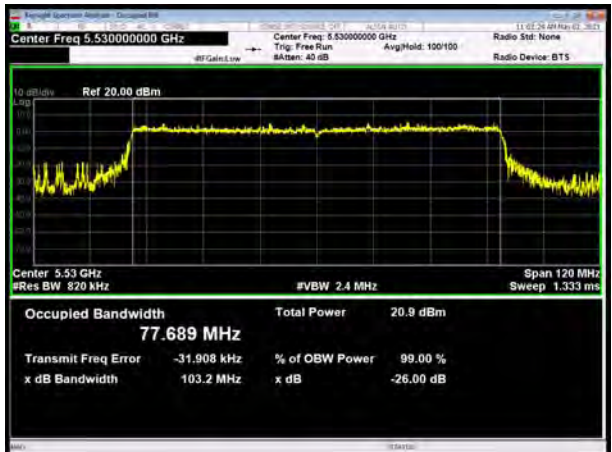
U-NII-2C, 802.11ax HE80 SU Mode 996-Tones, Carrier frequency (MHz): 5690
