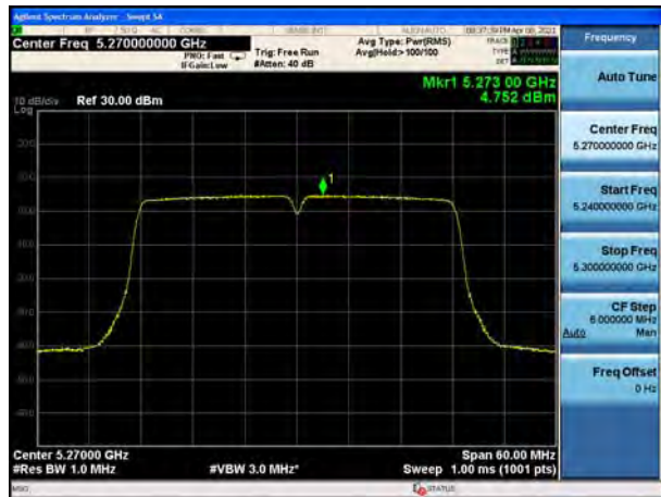
U-NII-2A, 802.11ac VHT40, Channel No.: 54
