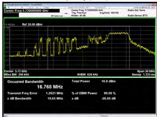
U-NII-2C, 802.11ax HE20 MU Mode 52-Tones, Carrier frequency (MHz): 5720
