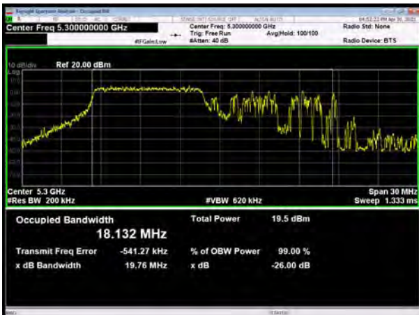
U-NII-2A, 802.11ax HE20 MU Mode 106-Tones, Carrier frequency (MHz): 5320
