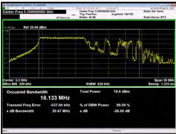
U-NII-1, 802.11ax HE20 MU Mode 106-Tones, Carrier frequency (MHz): 5200
