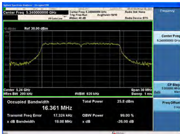
U-NII-1, 802.11a Carrier frequency (MHz): 5240
