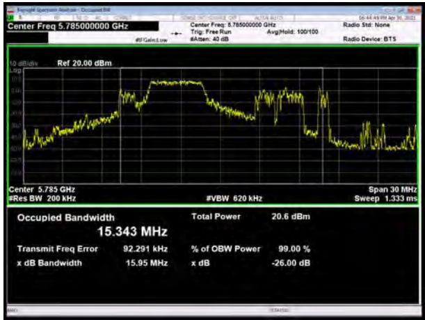
U-NII-3, 802.11ax HE20 MU Mode 52-Tones, Carrier frequency (MHz): 5785
