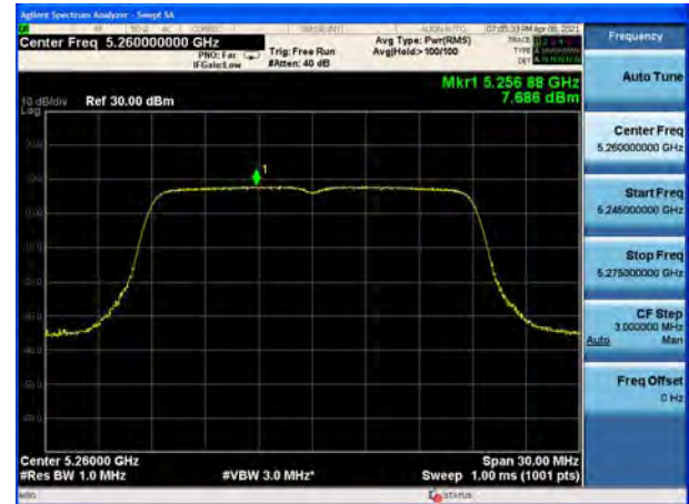
U-NII-2A, 802.11ac VHT20, Channel No.: 60
