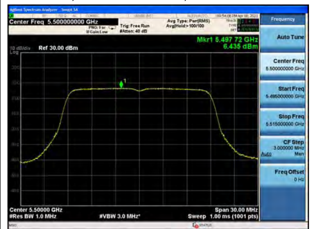
U-NII-2C, 802.11ac VHT20, Channel No.: 116
