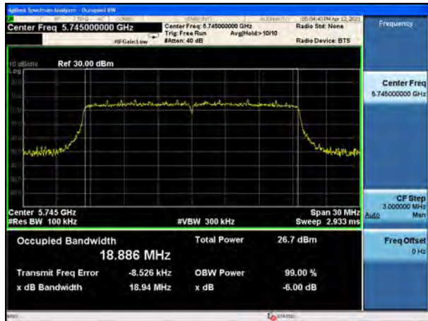
U-NII-3, 802.11ax HE20 Carrier frequency (MHz): 5745
