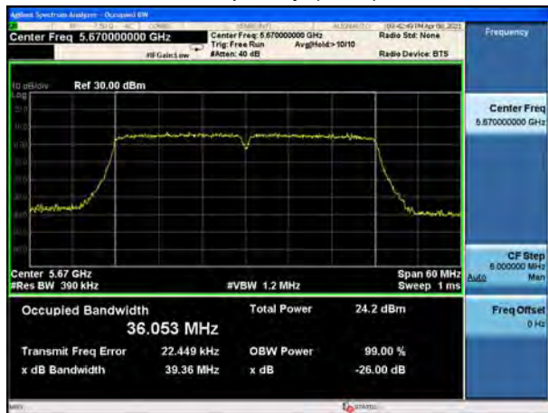
U-NII-2C, 802.11n HT40 Carrier frequency (MHz): 5670
