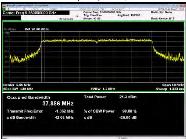
U-NII-2C, 802.11ax HE40 SU Mode 484-Tones, Carrier frequency (MHz): 5550
