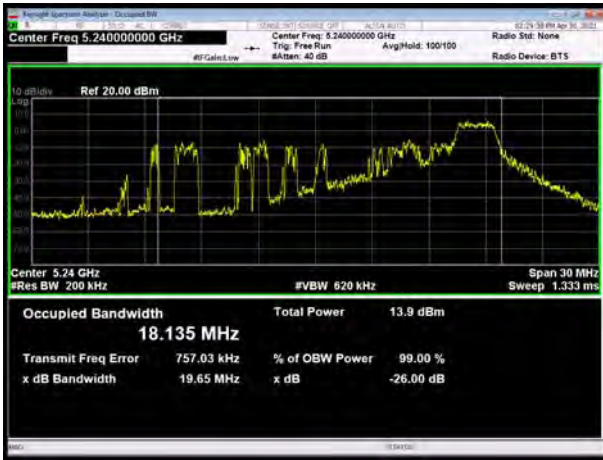
U-NII-1, 802.11ax HE20 MU Mode 26-Tones, Carrier frequency (MHz): 5240
