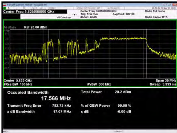
U-NII-3, 802.11ax HE40 SU Mode 484-Tones, Carrier frequency (MHz): 5755
