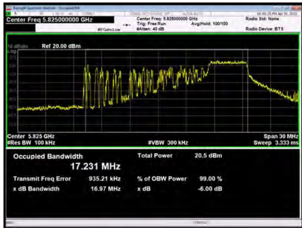
U-NII-3, 802.11ax HE20 MU Mode 52-Tones, Carrier frequency (MHz): 5825
