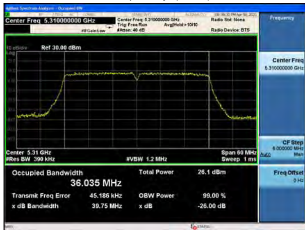
U-NII-2A, 802.11ax HE20 Carrier frequency (MHz): 5260
