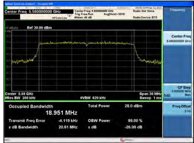
U-NII-2C, 802.11ax HE20 Carrier frequency (MHz):5720
