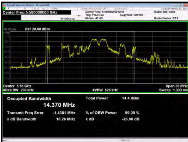
U-NII-2C, 802.11ax HE20 MU Mode 26-Tones, Carrier frequency (MHz): 5700
