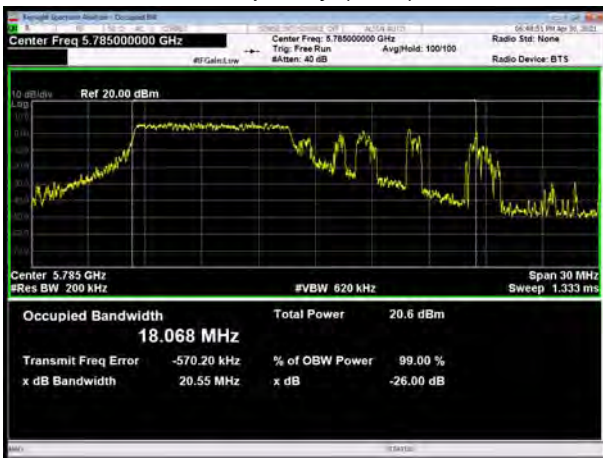
U-NII-3, 802.11ax HE20 MU Mode 106-Tones, Carrier frequency (MHz): 5785
