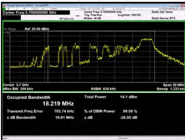
U-NII-2C, 802.11ax HE20 MU Mode 26-Tones, Carrier frequency (MHz): 5720
