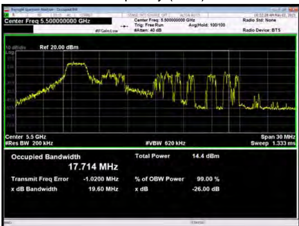
U-NII-2C, 802.11ax HE20 MU Mode 26-Tones, Carrier frequency (MHz): 5500
