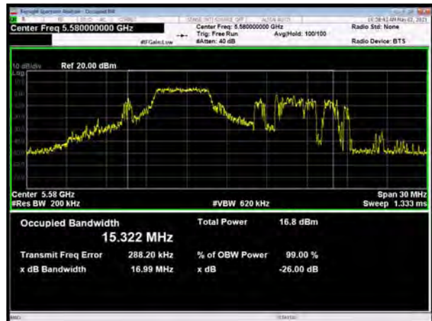
U-NII-2C, 802.11ax HE20 MU Mode 52-Tones, Carrier frequency (MHz): 5700
