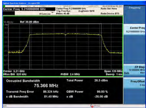
U-NII-1, 802.11ax HE40 Carrier frequency (MHz): 5190
