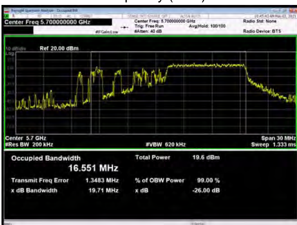
U-NII-2C, 802.11ax HE20 MU Mode 106-Tones, Carrier frequency (MHz): 5700
