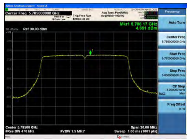
U-NII-3, 802.11ac VHT20, Channel No.: 157
