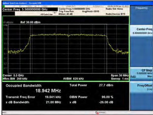
U-NII-2C, 802.11ax HE20 Carrier frequency (MHz):5700
