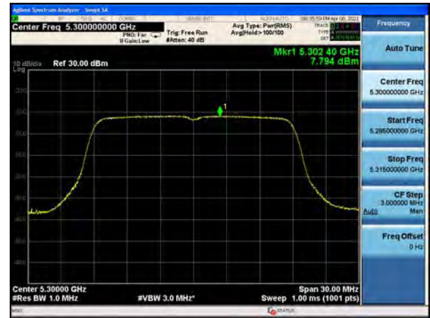
U-NII-2A, 802.11ac VHT20, Channel No.: 60
