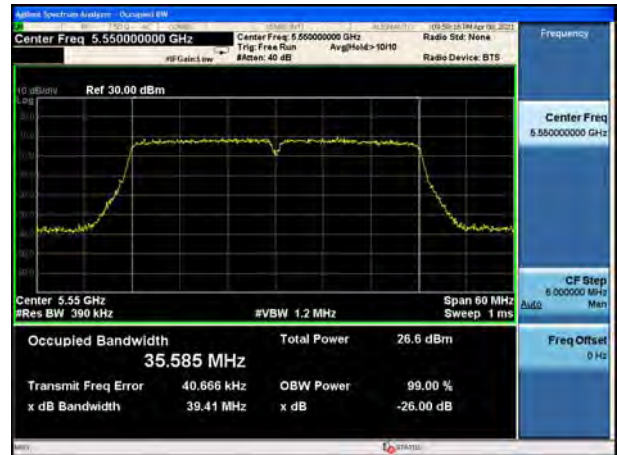
U-NII-2C, 802.11ax HE40 Carrier frequency (MHz): 5550
