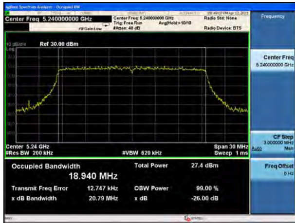
U-NII-1, 802.11ax HE20 Carrier frequency (MHz): 5240
