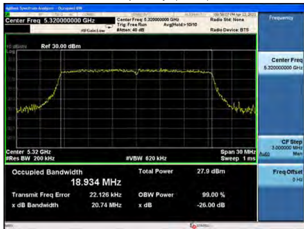
U-NII-2A, 802.11ax HE20 Carrier frequency (MHz): 5320
