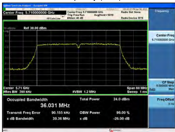
U-NII-2C, 802.11n HT40 Carrier frequency (MHz): 5710
