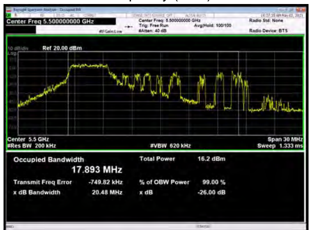
U-NII-2C, 802.11ax HE20 MU Mode 52-Tones, Carrier frequency (MHz): 5500
