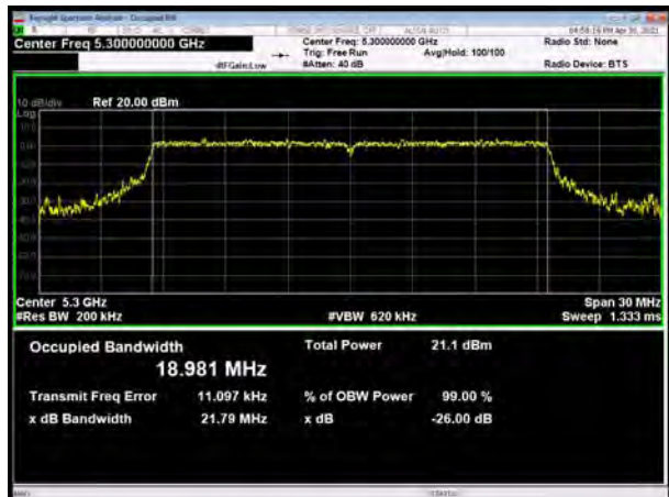
U-NII-2A, 802.11ax HE20 SU Mode 242-Tones, Carrier frequency (MHz): 5320
