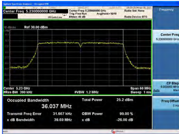
U-NII-1, 802.11ax HE20 Carrier frequency (MHz): 5180
