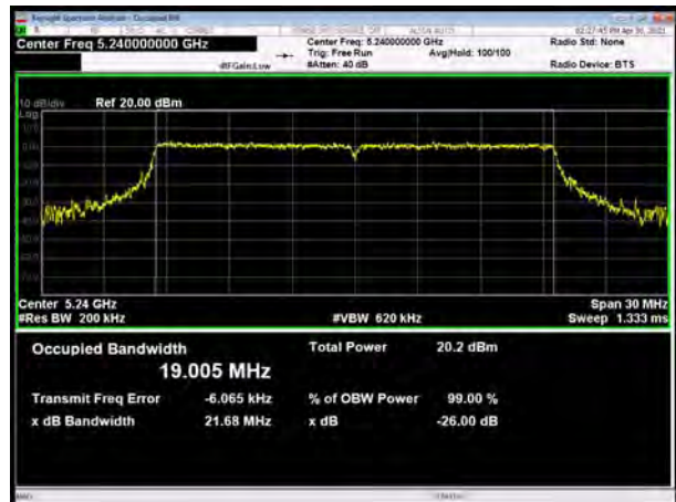
U-NII-1, 802.11ax HE80 SU Mode 996-Tones, Carrier frequency (MHz): 5210
