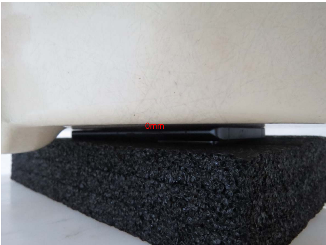
Picture 14: Front Side, the distance from handset to the bottom of the Phantom is 0mm
