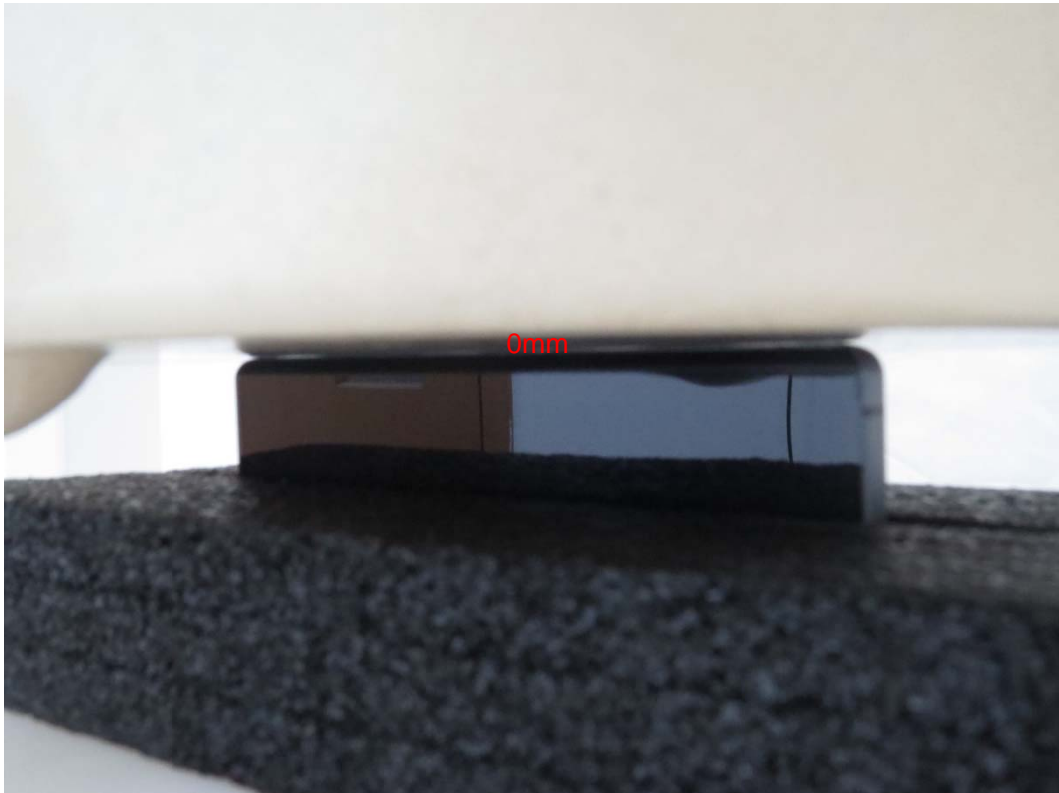
Picture 15: Left Side, the distance from handset to the bottom of the Phantom is 0mm
