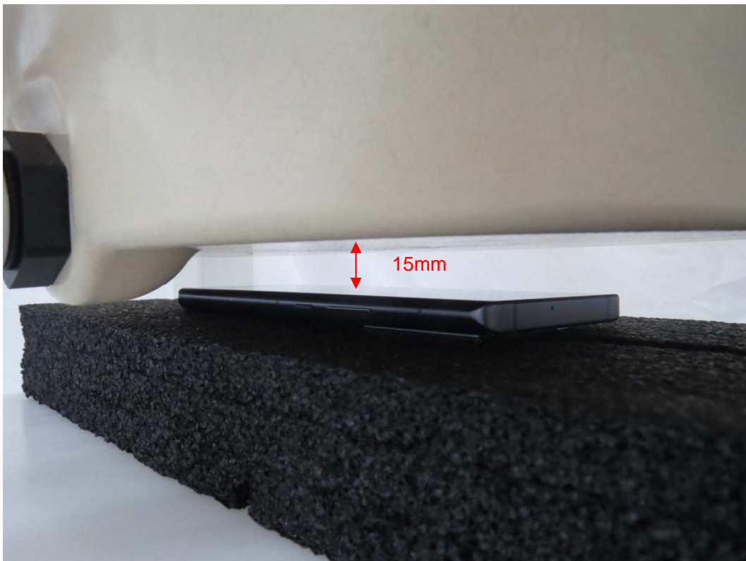
Picture 6: Front Side, the distance from handset to the bottom of the Phantom is 15mm
