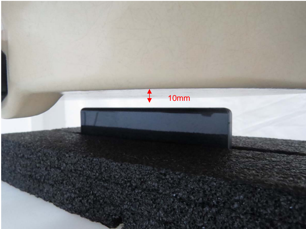
Picture 9: Left Side, the distance from handset to the bottom of the Phantom is 10mm
