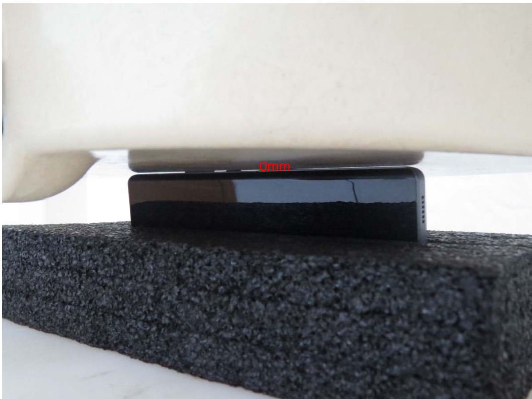
Picture 16: Right Side, the distance from handset to the bottom of the Phantom is 0mm
