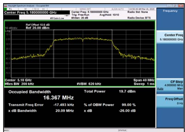
U-NII-1 26dB Bandwidth-802.11a(20MHz) ,5180MHz
