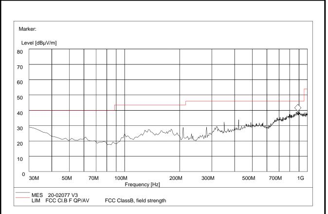
Plot B: 30MHz to 1GHz, Antenna Vertical
