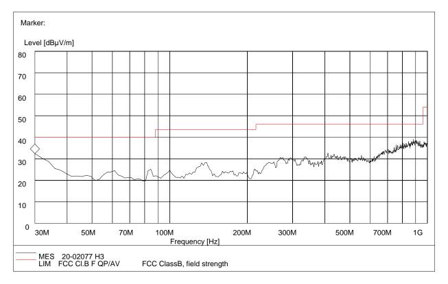
Plot A: 30MHz to 1GHz, Antenna Horizontal
