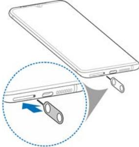
2. Pull out the card tray. You can place a nano-SIM card on the upper card slot, and place a microSDXC card (optional) on the lower card slot, as shown. Carefully slide the tray back into place.
