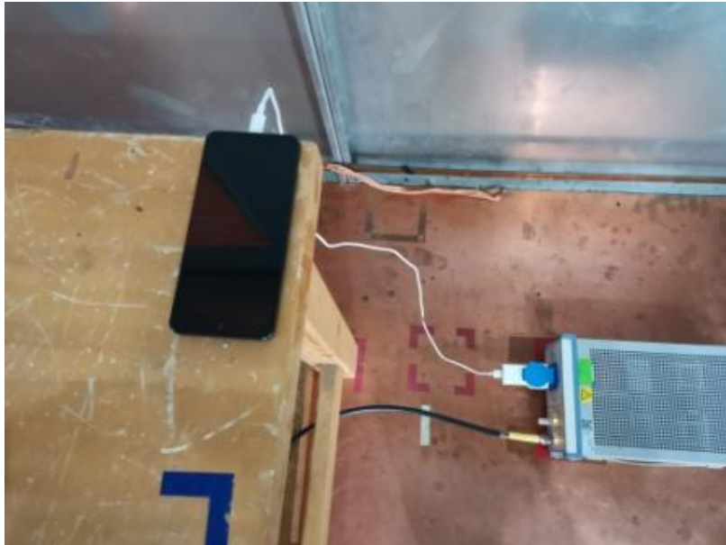
Conducted Emissions Test Setup (with charger)
