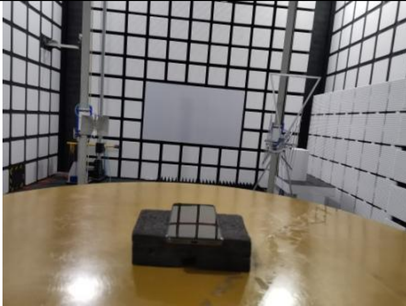
Spurious Radiated Emissions Test setup
