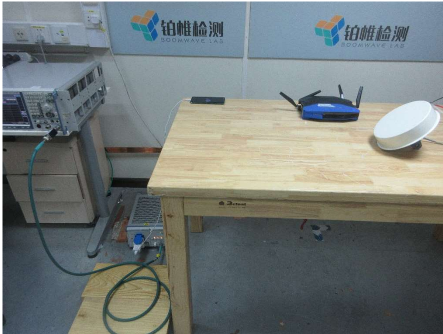
Conducted Emission 150kHz-30MHz (Front view) – Mode 2
