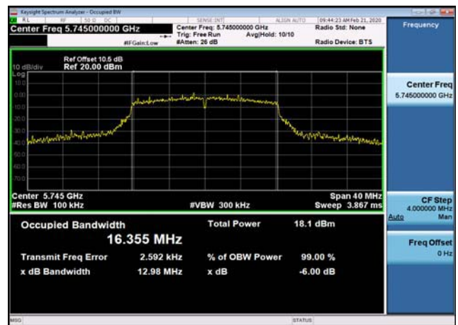
U-NII-3 6dB Bandwidth-802.11a(20MHz) ,5825MHz,Ant1
