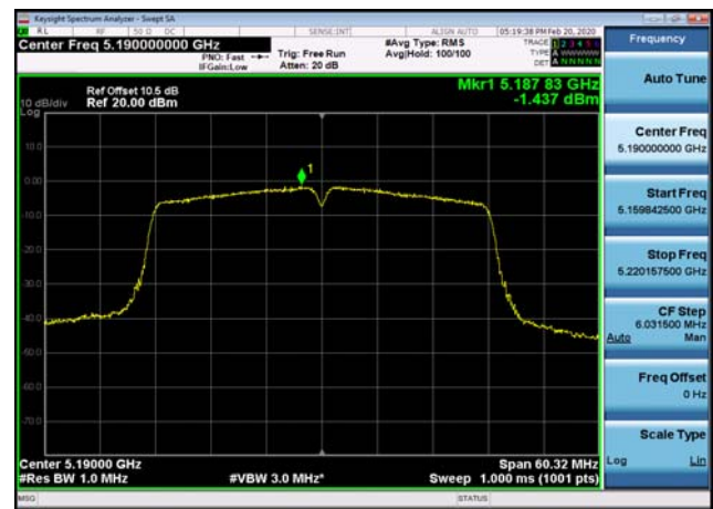
U-NII-1 Power spectral density-802.11 ac(40MHz),5190MHz
