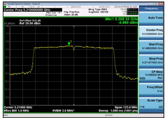
U-NII-3 Power spectral density-802.11 n(20MHz),5785MHz
