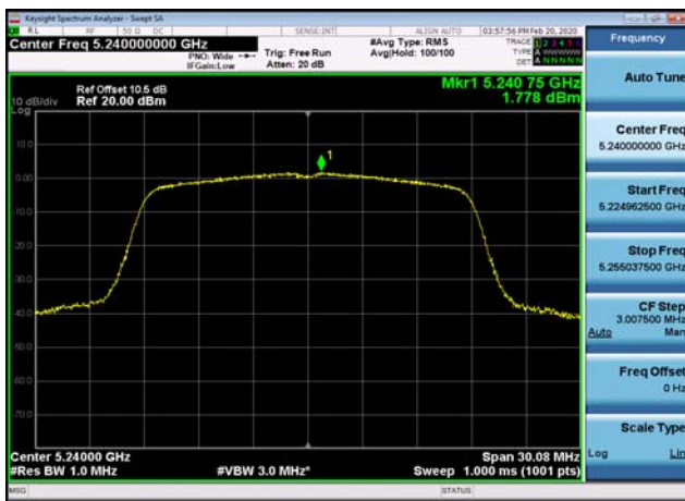
U-NII-1 Power spectral density-802.11 ac(20MHz),5240MHz
