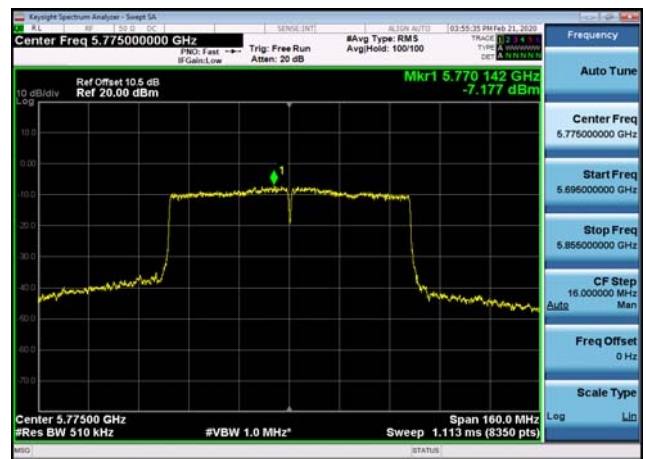
U-NII-3 Power spectral density-802.11 ac(80MHz),5775MHz
