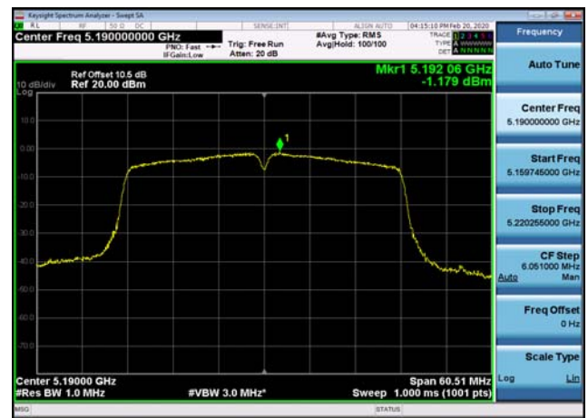
U-NII-1 Power spectral density-802.11 a(20MHz),5180MHz
