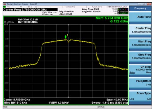
U-NII-3 Power spectral density-802.11 n(40MHz),5755MHz
