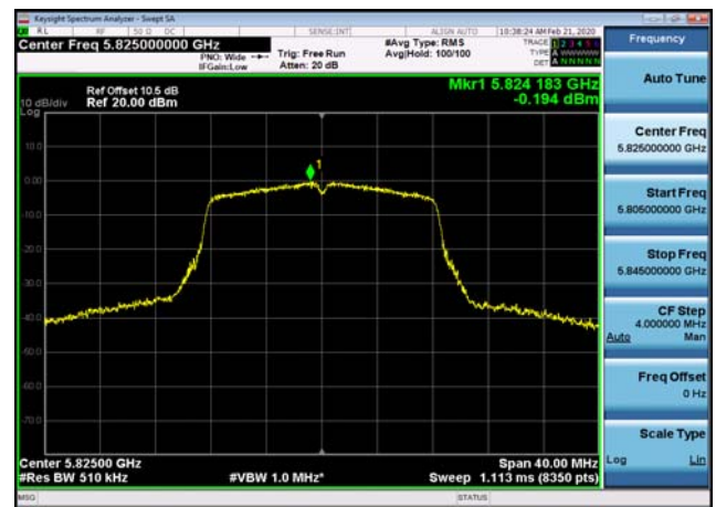
U-NII-3 Power spectral density-802.11 ac(20MHz),5785MHz
