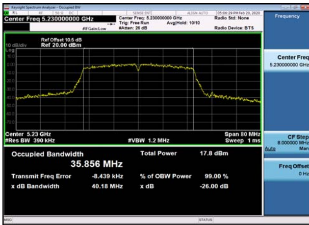
U-NII-3 6dB Bandwidth-802.11n(20MHz),5745MHz,Ant1
