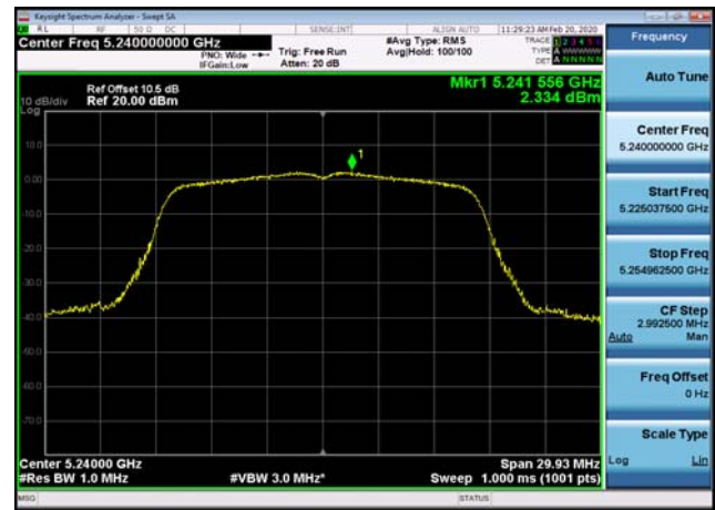
U-NII-1 Power spectral density-802.11 ac(20MHz),5220MHz
