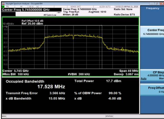
U-NII-3 6dB Bandwidth-802.11n(20MHz),5825MHz,Ant1
