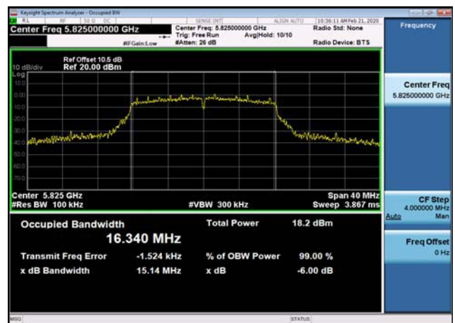
U-NII-3 6dB Bandwidth-802.11ac(20MHz) ,5785MHz,Ant1
