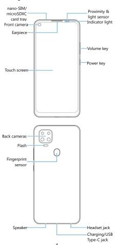
**Setting Up Your Phone**The nano-SIM card can be installed or removed while the phone is turned on.
