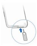
Pull out the card tray and place the nano-SIM card and the microSDXC card (optional) on the tray, as shown. Carefully slide the tray back into place.
