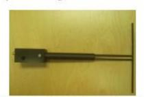
Figure 1 – MVG COMOSAR Validation Dipole
