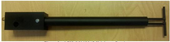
Figure 1 – MVG COMOSAR Validation Dipole
