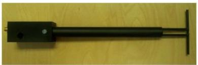
Figure 1 - MVG COMOSAR Validation Dipole
