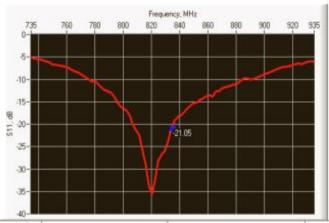
Frequency (MHz) Return Loss (dB) Requirement (dB) Impedance 835 -21.05 -20  $59.7 \Omega + 0.2 \text{ j}\Omega$
