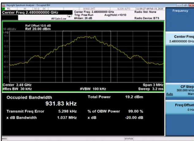
20dB Bandwidth: DQPSK,2441MHz,2DH5
