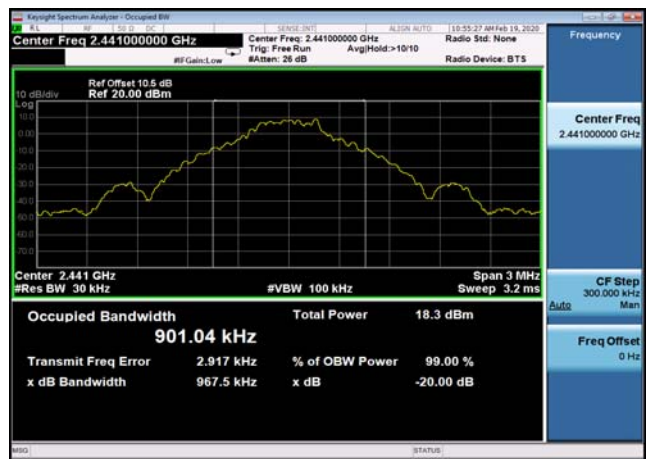
20dB Bandwidth: DQPSK,2402MHz,2DH5
