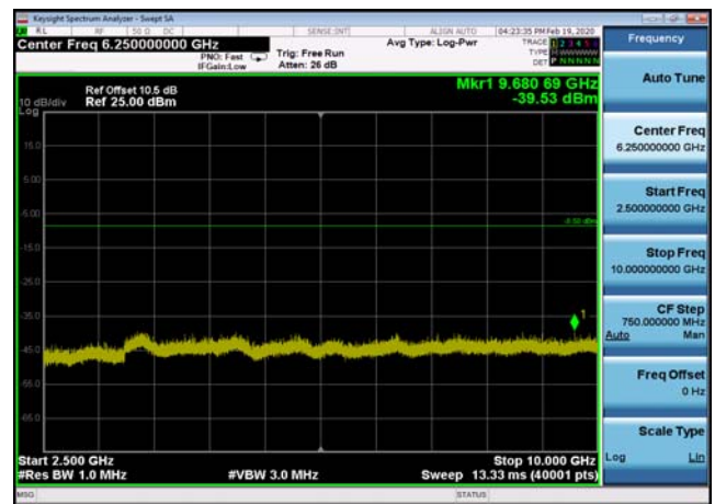
Conducted Emission: 8DPSK,2480,3DH5 ,2500MHz~10000MHz
