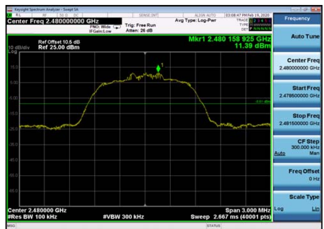
Conducted Emission: DQPSK,2480,2DH5 ,Reference Level
