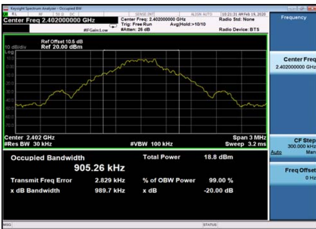
20dB Bandwidth: GFSK,2480MHz,DH5
