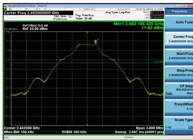
Conducted Emission: GFSK,2402,DH5 ,Reference Level
