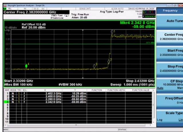
Conducted Emission: 8DPSK,2402,3DH5 ,Band Edge
