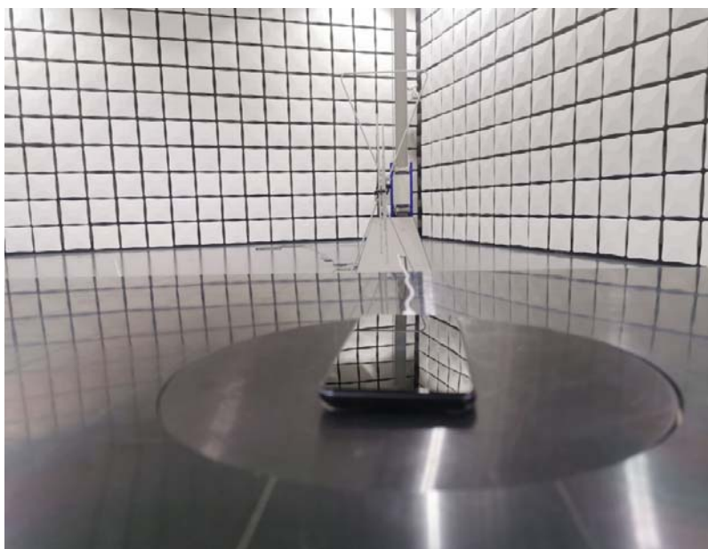
RF Conducted Test setup (BT/WIFI)
