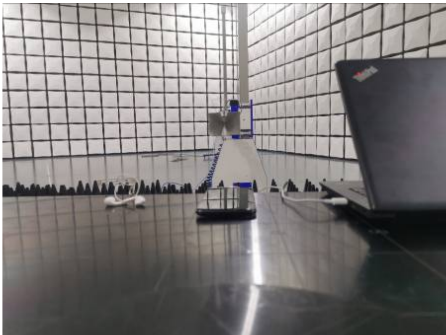
Radiated Emissions Test Setup (above 1GHz)
