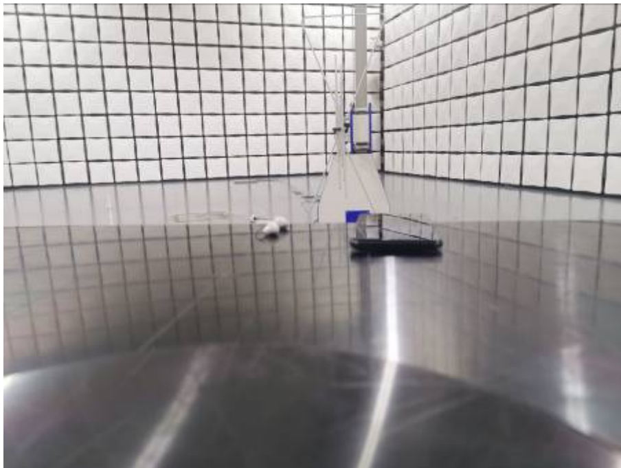
Radiated Emissions Test Setup (30-1000MHz)
