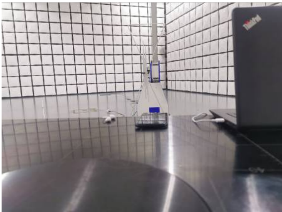
Radiated Emissions Test Setup (30-1000MHz)
