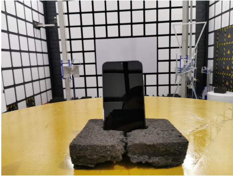
Spurious Radiated Emissions Test setup
