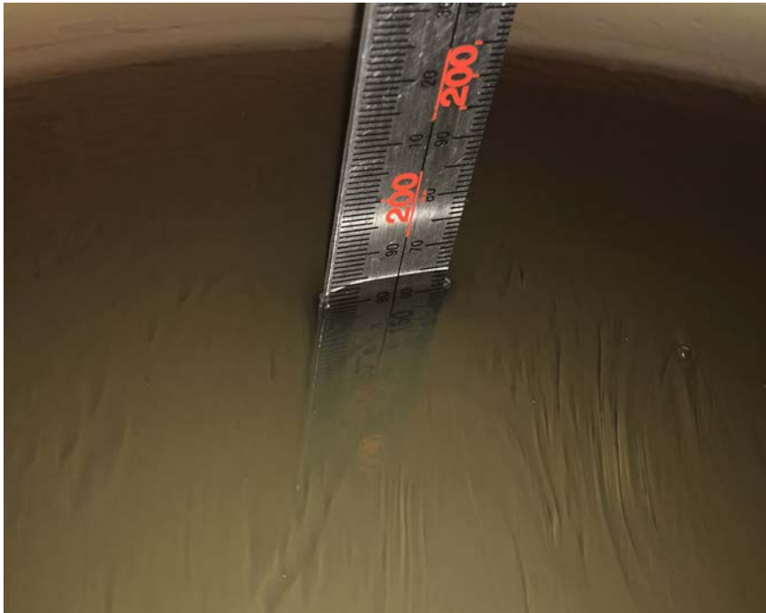
Liquid depth for SAR Measurement
