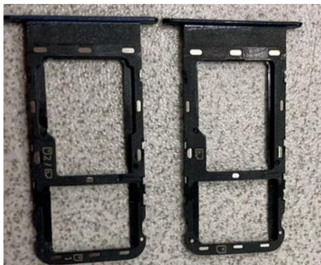
Figure: Double card tray on the left, single card tray on the right.
