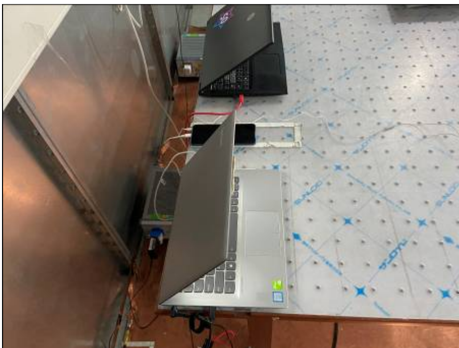
Conducted Emissions Test Setup (with laptop)
