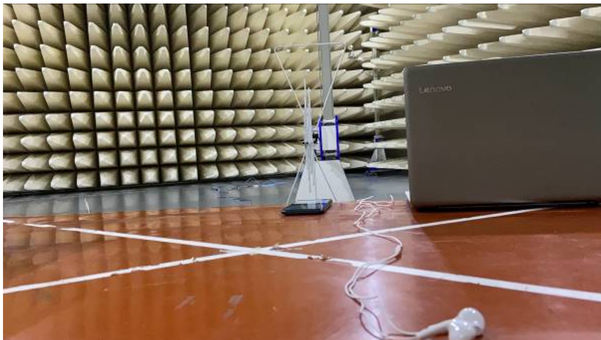
Radiated Emissions Test Setup (with laptop) (30-1000MHz)
