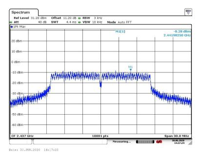
Carrier frequency (MHz): 2437 Channel No.6 Test Mode: 802.11g
