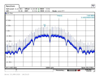
Carrier frequency (MHz): 2437 Channel No.6 Test Mode: 802.11b
