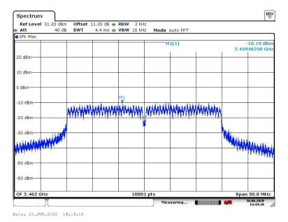
Carrier frequency (MHz): 2462 Channel No.11 Test Mode: 802.11n (HT20)
