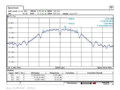
Carrier frequency (MHz): 2462 Channel No.:11 Test Mode: 802.11b
