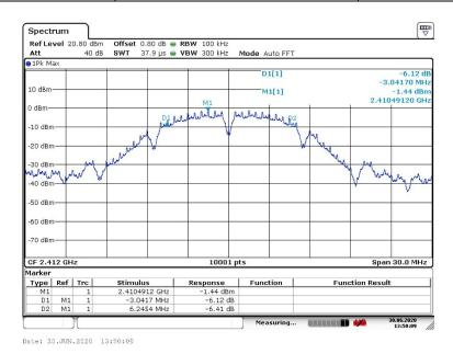
Carrier frequency (MHz): 2412 Channel No.:1
