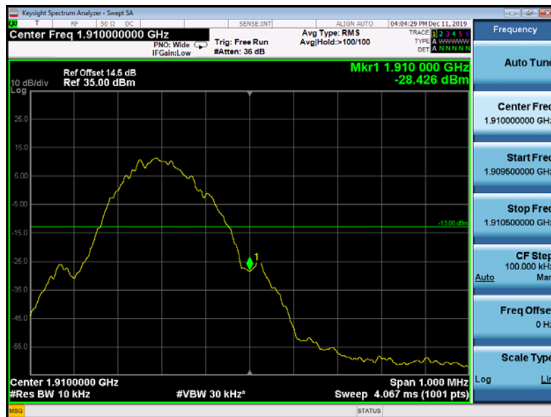
(Plot D: GSM 1900 Channel = 810)
