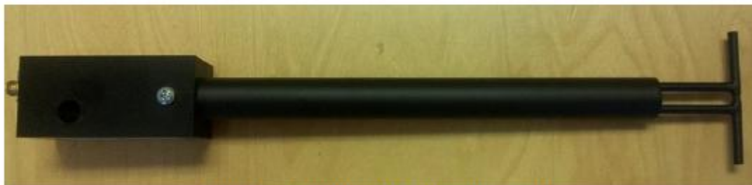
Figure 1 – MVG COMOSAR Validation Dipole
