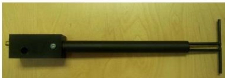
Figure 1 – MVG COMOSAR Validation Dipole
