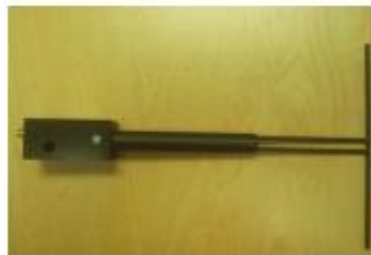
Figure 1 – MVG COMOSAR Validation Dipole
