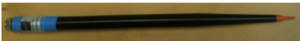
Figure 1 – MVG COMOSAR Dosimetric E field Dipole
