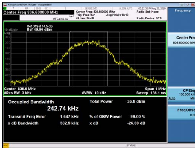
(Plot C2: EDGE 850MHz Channel = 190 Occupied bandwidth)
