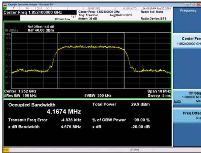
(Plot F1: WCDMA 1900MHz Channel = 9262 Occupied bandwidth)
