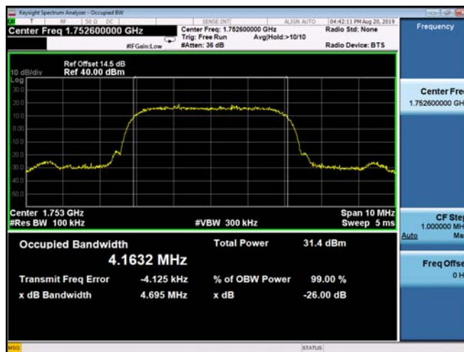
(Plot G2: WCDMA 1700MHz Channel = 1412 Occupied bandwidth)
