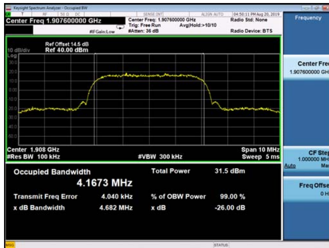
(Plot F2: WCDMA 1900MHz Channel = 9400 Occupied bandwidth)
