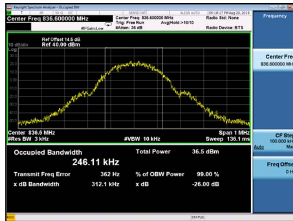
(Plot A2: GSM 850MHz Channel = 190 Occupied bandwidth)
