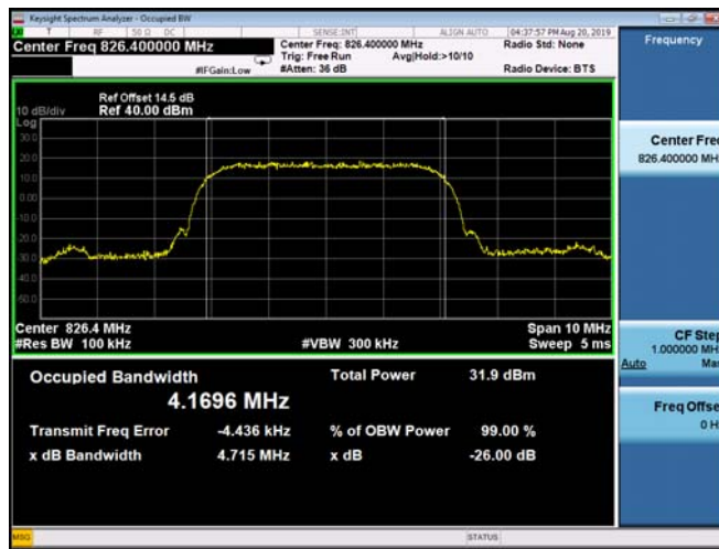
(Plot E1: WCDMA 850MHz Channel = 4132 Occupied bandwidth)
