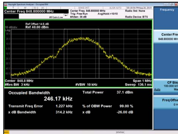
(Plot A3: GSM 850MHz Channel = 251 Occupied bandwidth)
