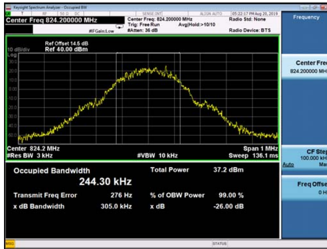
(Plot C1: EDGE 850MHz Channel = 128 Occupied bandwidth)
