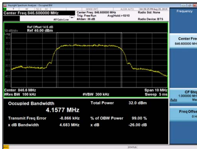
(Plot E2: WCDMA 850MHz Channel = 4183 Occupied bandwidth)
