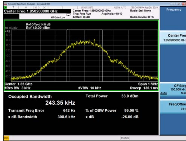
(Plot B1: GSM 1900MHz Channel = 512 Occupied bandwidth)
