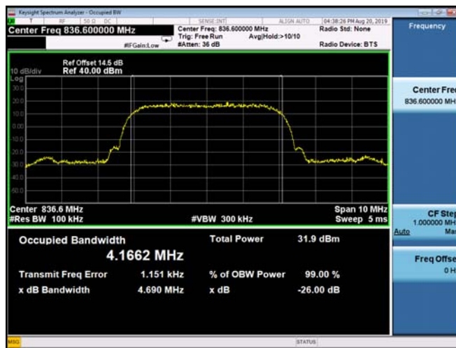
(Plot E2: WCDMA 850MHz Channel = 4183 Occupied bandwidth)
