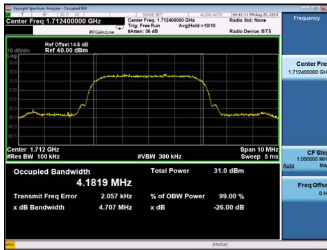
(Plot G1: WCDMA 1700MHz Channel = 1312 Occupied bandwidth)
