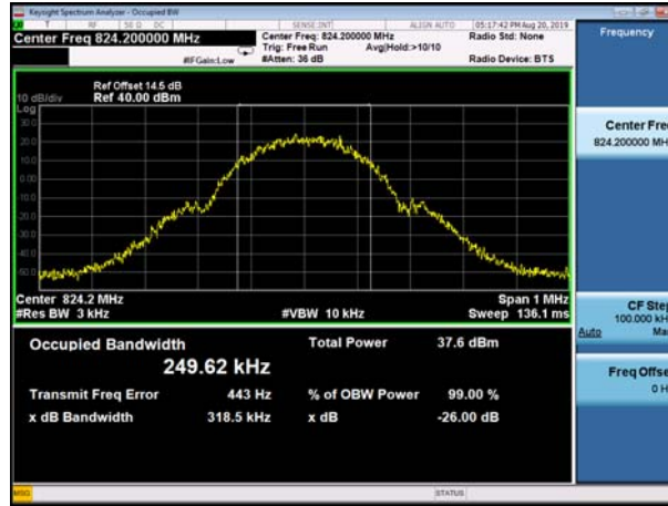
(Plot A1: GSM 850MHz Channel = 128 Occupied bandwidth)
