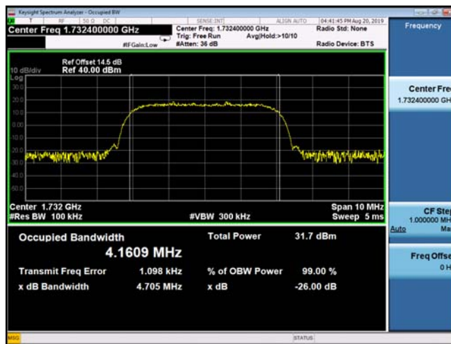
(Plot G2: WCDMA 1700MHz Channel = 1412 Occupied bandwidth)
