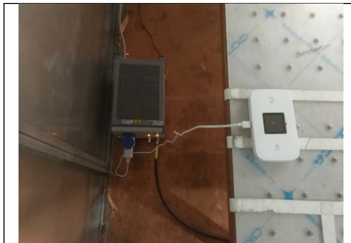
Conducted Emissions Test Setup (with charger)
