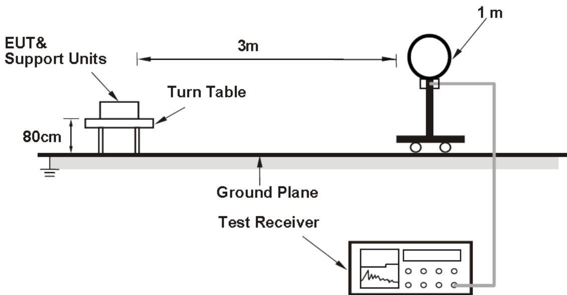
For Radiated emission 30MHz to 1GHz
