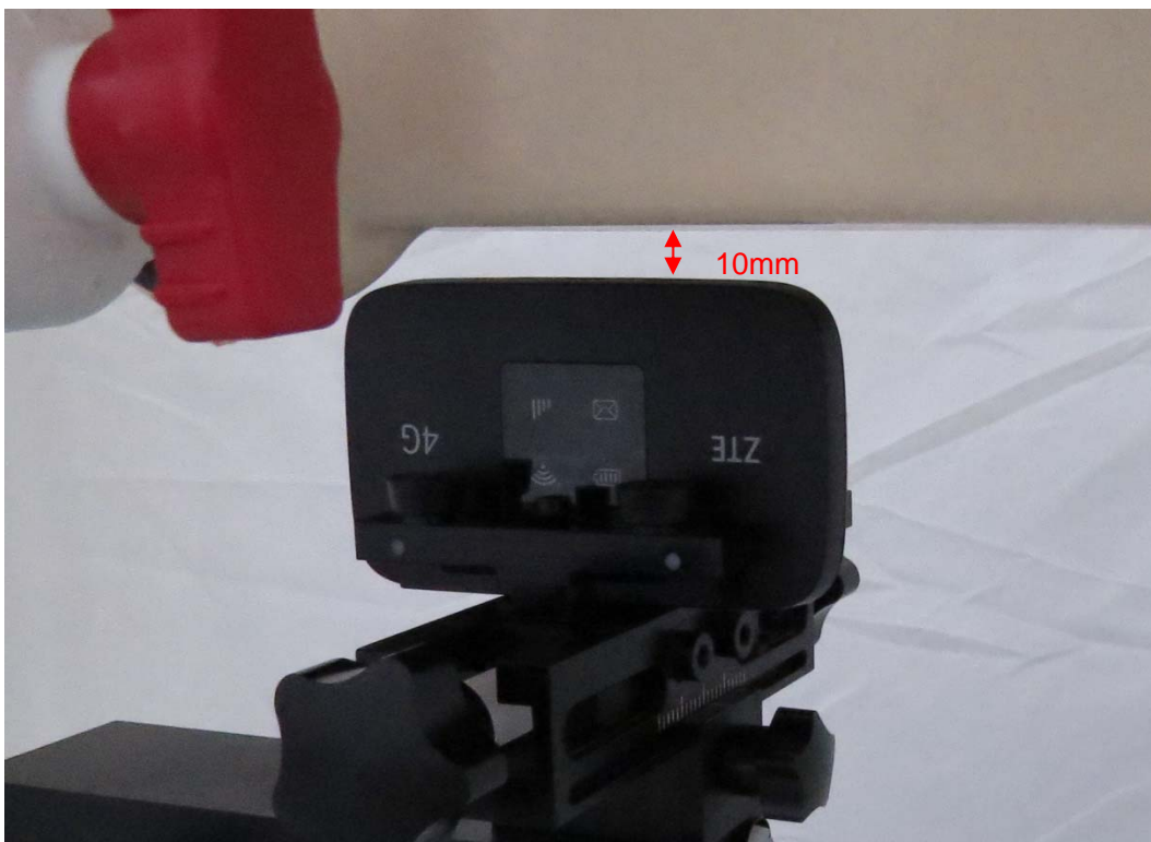
Picture 6: Bottom Side, the distance from handset to the bottom of the Phantom is 10mm
