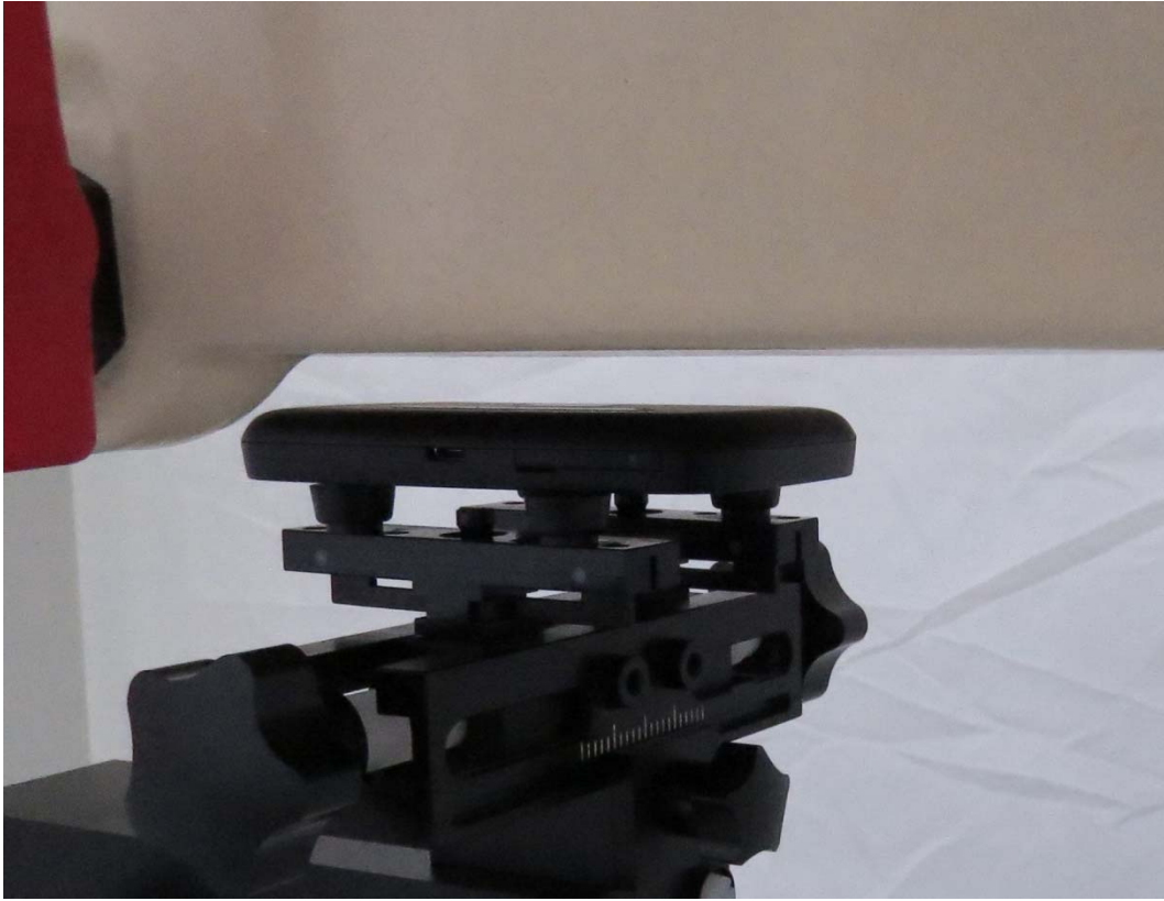
Picture 1: Back Side, the distance from handset to the bottom of the Phantom is 10mm
