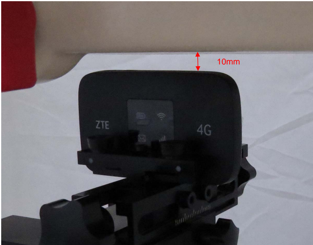
Picture 5: Top Side, the distance from handset to the bottom of the Phantom is 10mm
