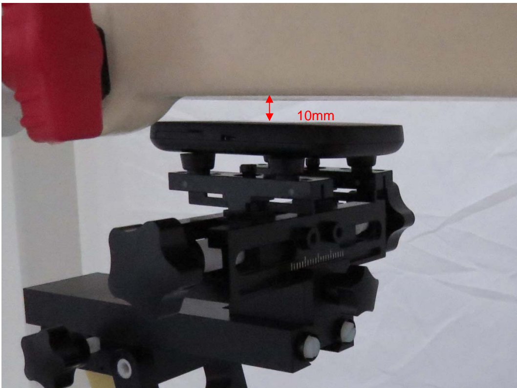
Picture 2: Front Side, the distance from handset to the bottom of the Phantom is 10mm
