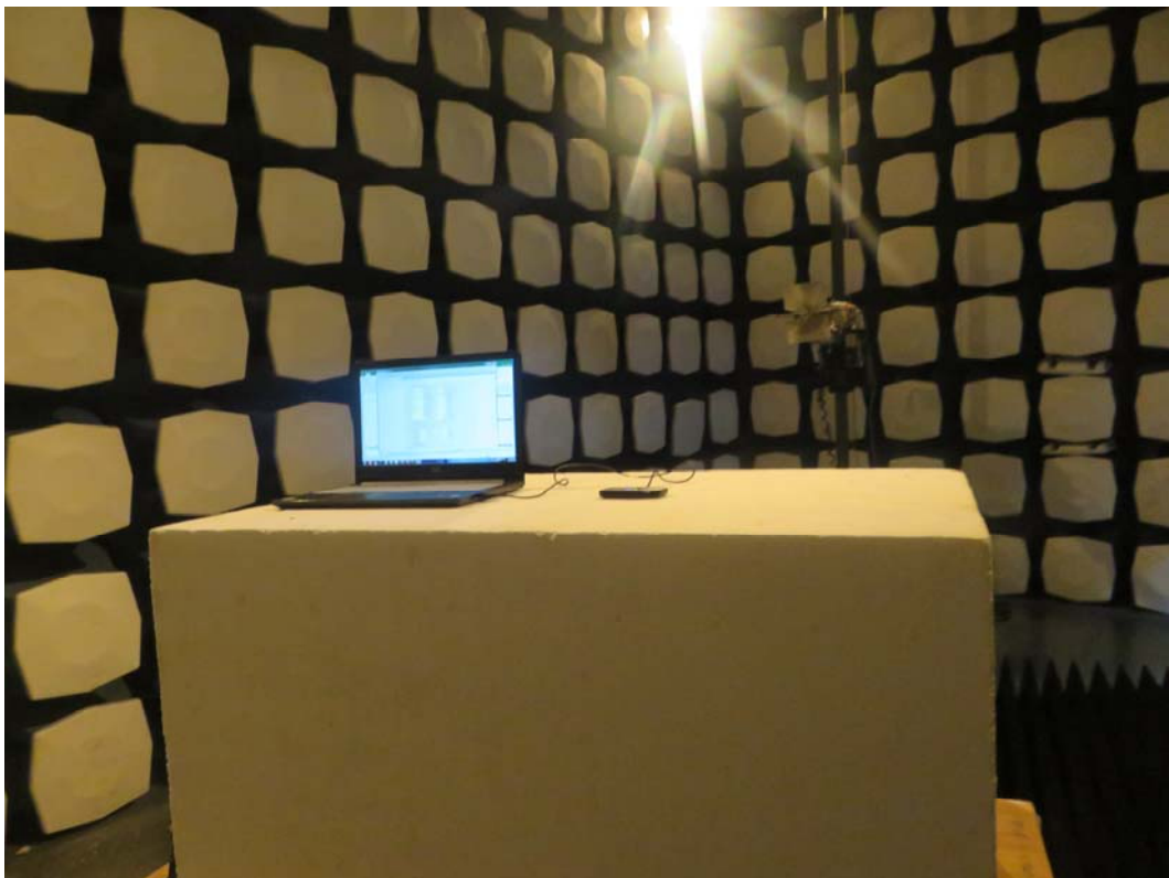
Picture 1: Radiated Spurious Emissions Test setup
