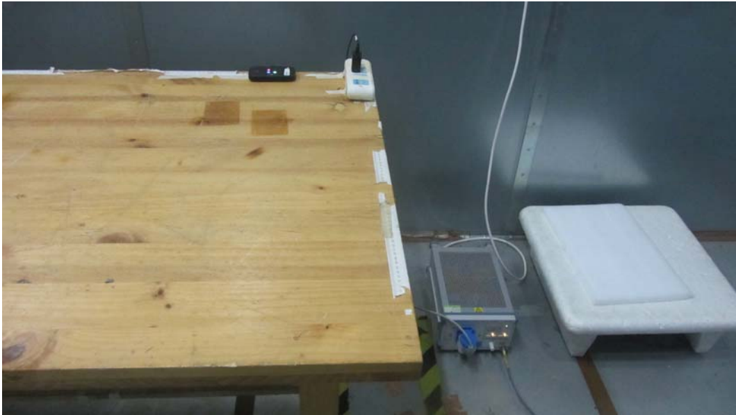
Picture 3 Conducted Emission Test Setup
