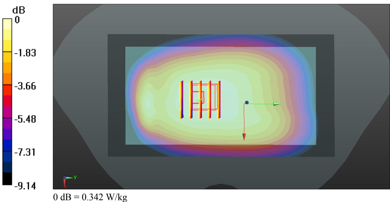
**16\_LTE Band 4\_20M\_QPSK\_1RB\_49Offset\_Back\_10mm\_Ch20175**
