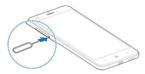
Place the nano-SIM card and the microSDXC card on the tray with the gold-colored contacts facing down.
