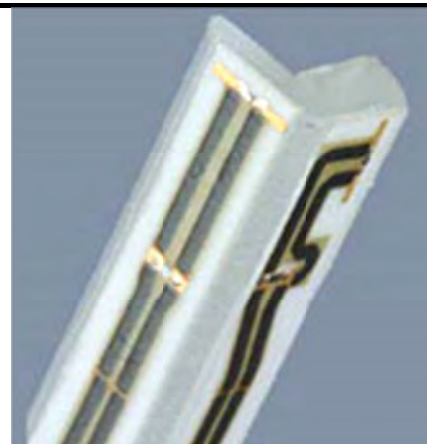
Fig 5.2 Photo of E-field Probe
