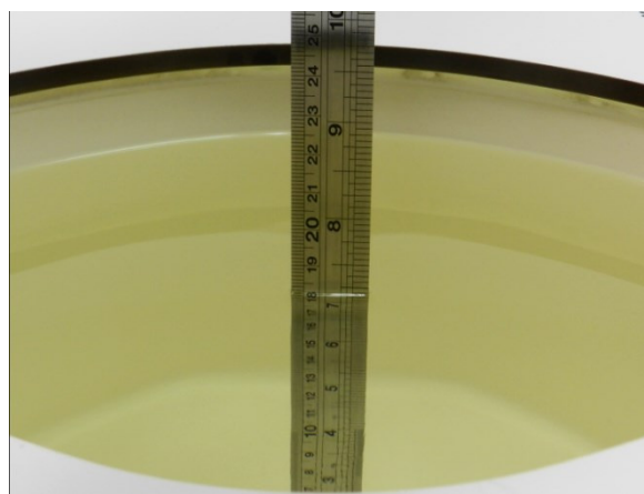
Fig 10.2 Photo of Liquid Height for Body SAR
