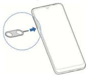
Pull out the card tray and place the nano-SIM card and the microSDXC card on the tray, as shown. Carefully slide the tray back into place.
