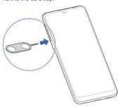
Pull out the card tray and place the nano-SIM card(s) and the microSDXC card on the tray, as shown. Carefully slide the tray back into place.
