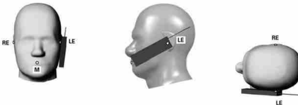
Fig 11.2.3 cheek or touch position. The reference points for the right ear (RE), left ear (LE), and mouth (M), which establish the Reference Plane for handset positioning, are indicated.
