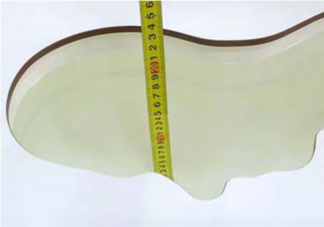
Picture 9: liquid depth in the head Phantom (1900 MHz, 15.3cm depth)
