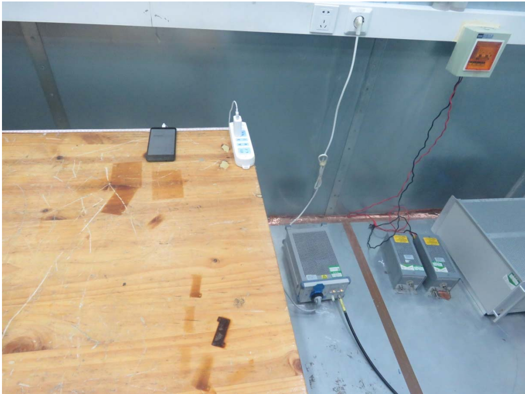
Picture 2 Conducted Emission Test Setup
