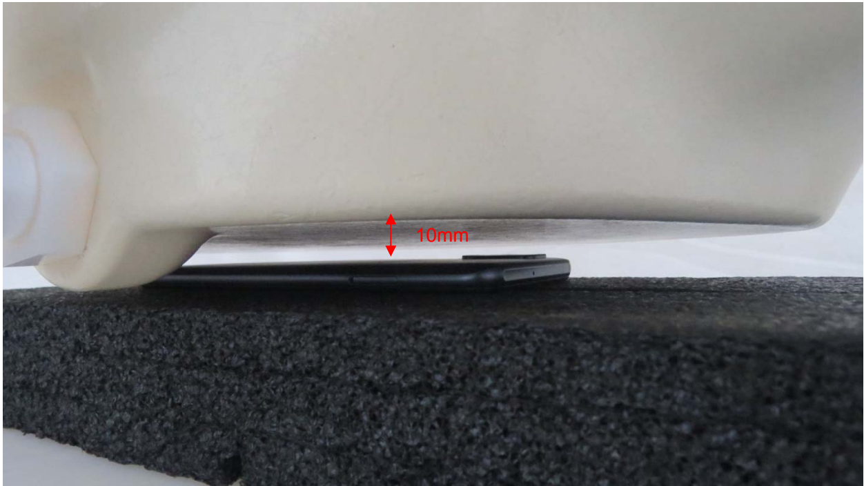
Picture 7: Back Side, the distance from handset to the bottom of the Phantom is 10mm
