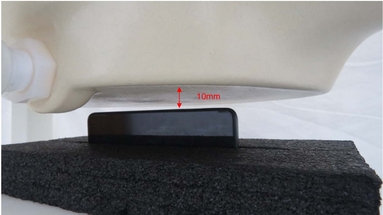
Picture 9: Left Side, the distance from handset to the bottom of the Phantom is 10mm
