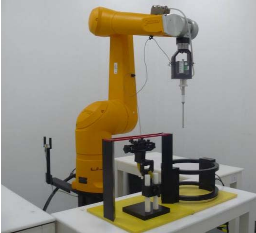
Picture 1: HAC T-Coil System Layout
