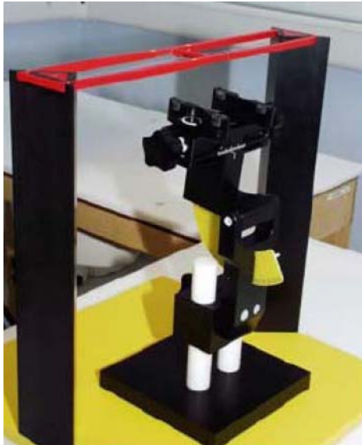
Figure 7 T-coil Phantom & Device Holder
