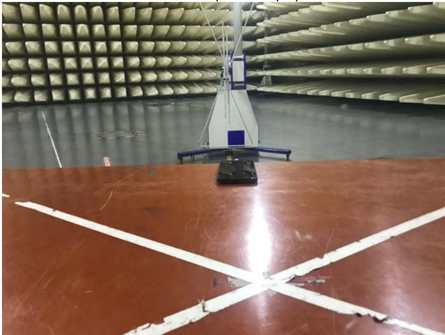
Radiated Emissions Test Setup (with charger) (30-1000MHz)
