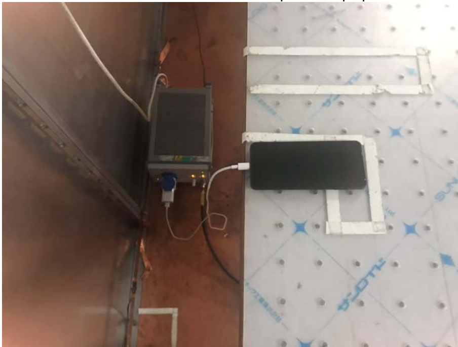
Conducted Emissions Test Setup (with charger)
