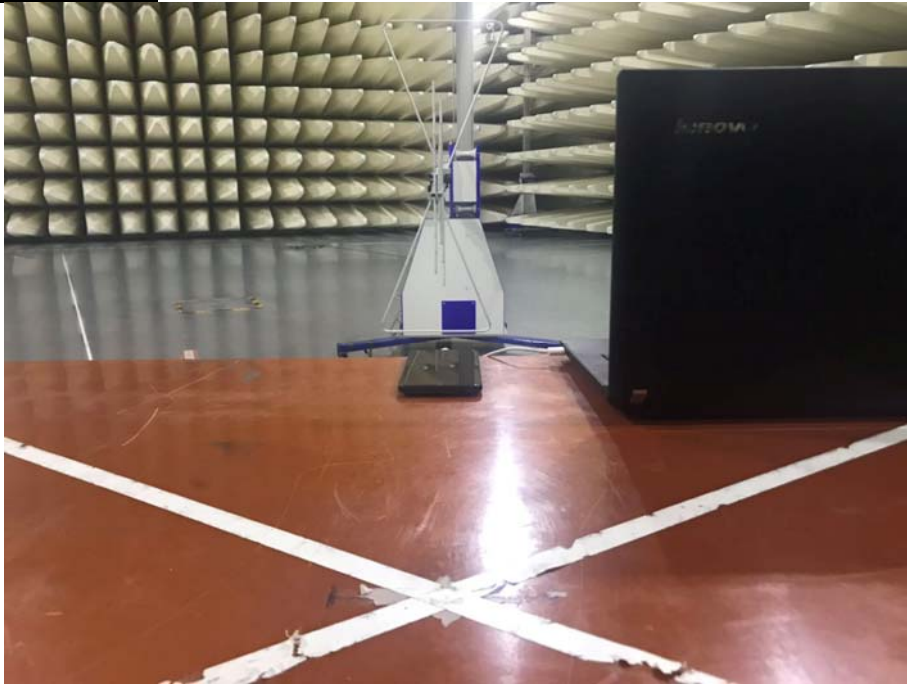
Radiated Emissions Test Setup (with laptop) (30-1000MHz)
