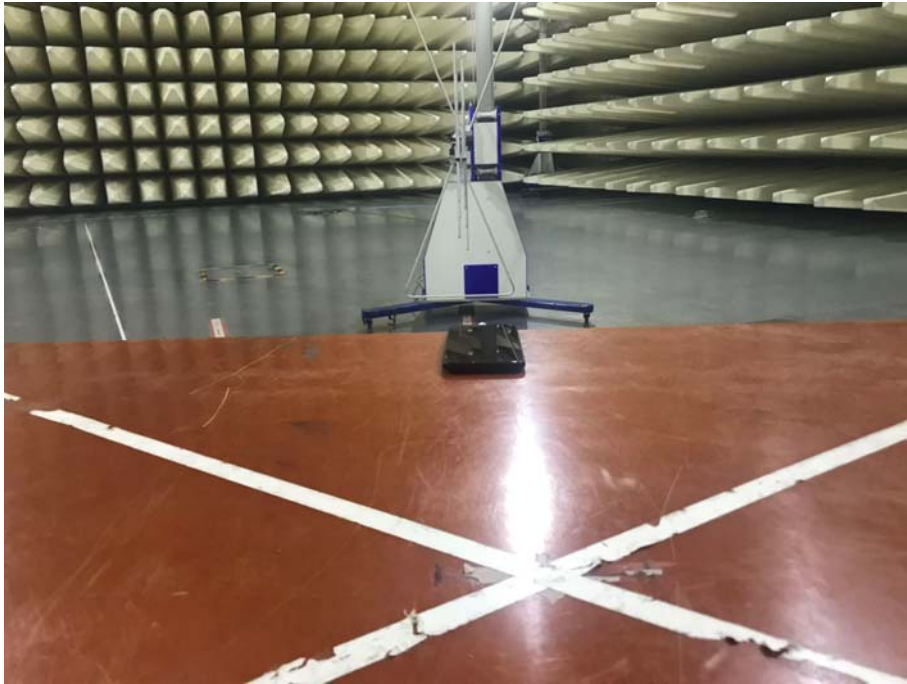
Radiated Emissions Test Setup(below 1GHz)
