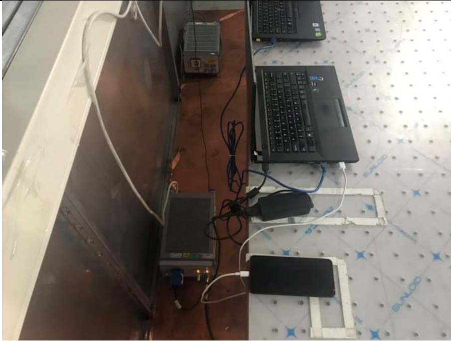
Conducted Emissions Test Setup (with laptop)
