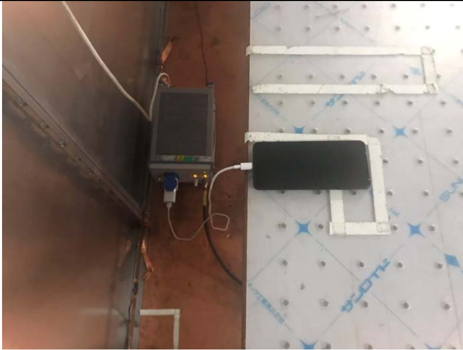
Conducted Emissions Test Setup (with charger)
