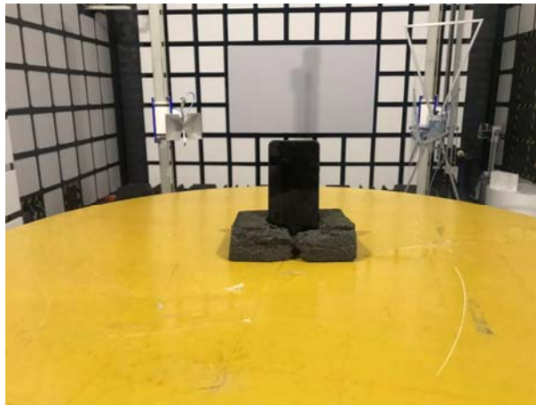
Conducted Emissions Test Setup (with charger)
