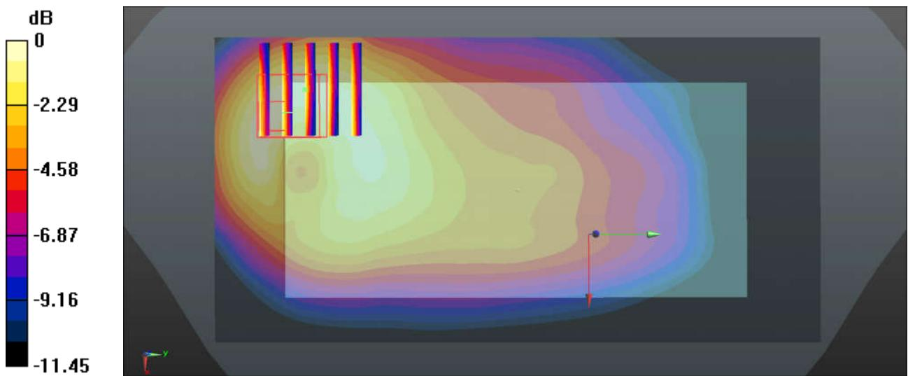
**37\_LTE Band 12\_10M\_QPSK\_1RB\_49Offset\_Back\_10mm\_Ch23095**
