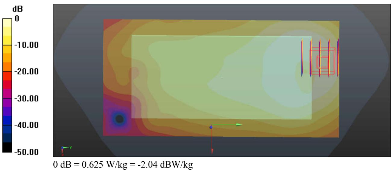
**26\_LTE Band66\_20M\_QPSK\_1RB\_0Offset\_Bottom Side\_10mm\_Ch132572**
