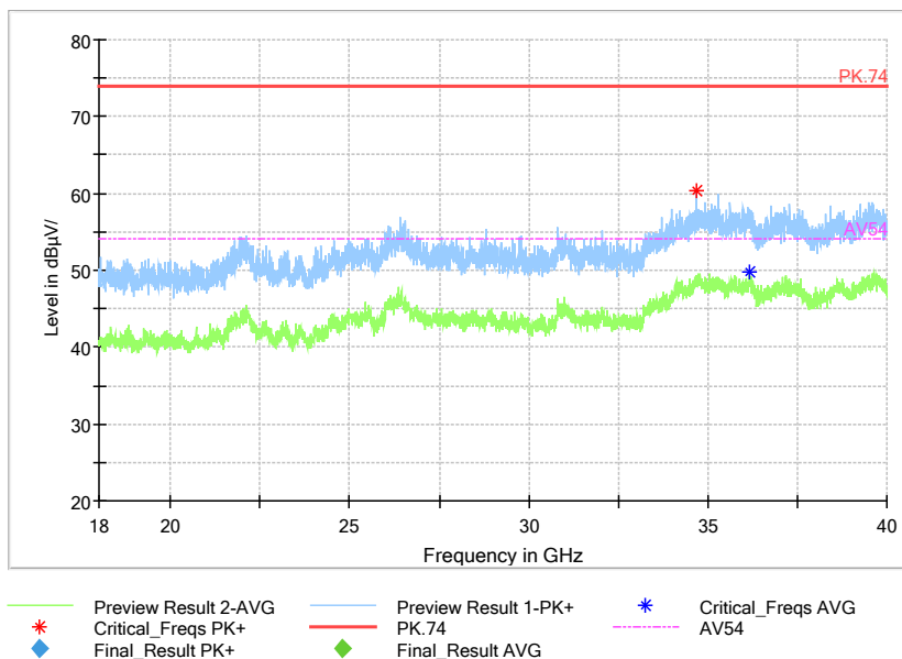
Pic9. Radiated emission (18GHz – 40GHz)
