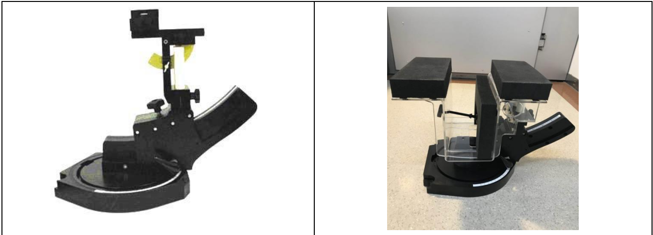
Device holder supplied by SPEAG
