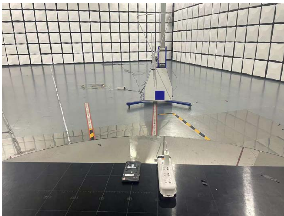
Radiated Emissions Test Setup (with charger) (30-1000MHz)
