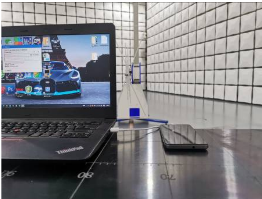
Radiated Emissions Test Setup (with laptop) (30-1000MHz)
