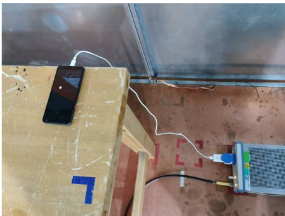
Conducted Emissions Test Setup (with charger)
