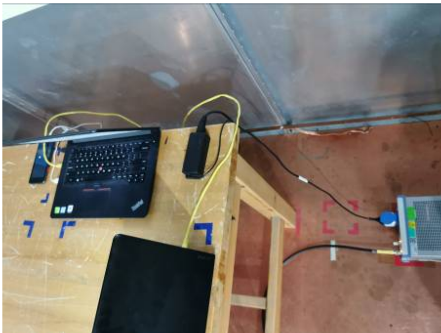
Conducted Emissions Test Setup (with laptop)
