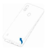
Insert the nano-SIM card and the optional microSDXC card into the correct card slots, as shown.
