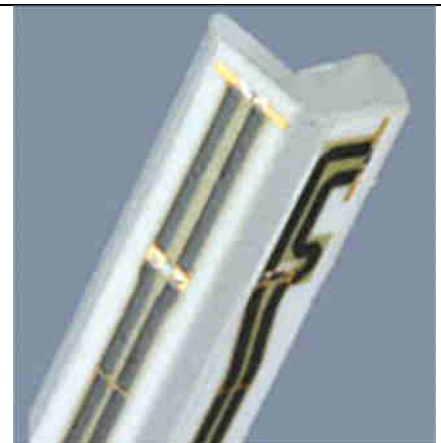
Fig 5.2 Photo of E-field Probe
