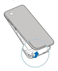
Install the nano-SIM card and the microSDXC card as shown.
