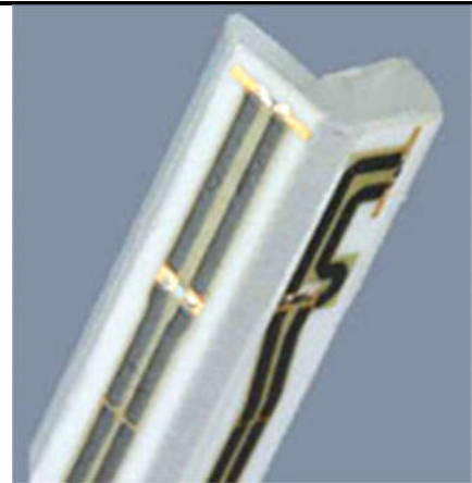
Fig 5.2 Photo of E-field Probe
